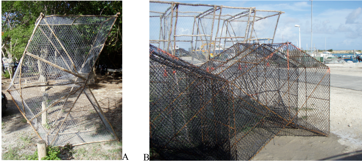
Figure 6 Lobsters and fish traps, with reinforcement out of A wood with wire-netting envelope, B metal with plastic envelope.
